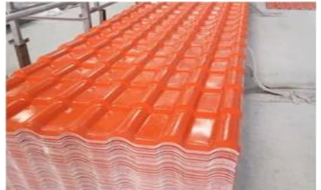
4. To achieve the length of customer needs cut off. after artificial out
