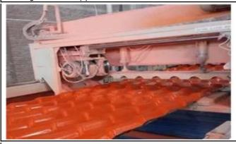
3. Then through the mold pressure, lastic the molding, cooling, throughthe traction machine slowly introduced
