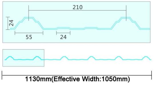
Model Number Type Overall Width Effective Width #1130-210-24 Trapezoid type 1130mm 1050mm
