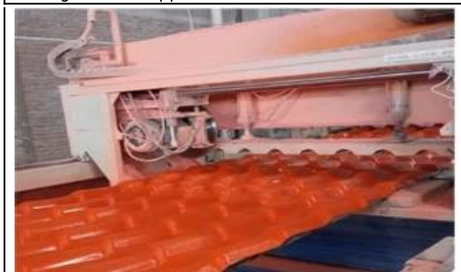
3. Then through the mold pressure, lactic the molding, cooling, through the traction machine slowly introduced
