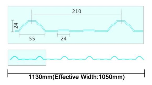
Model Number #1130-210-24 Trapezoid type Type Overall Width 1130mm Effective Width 1050mm
