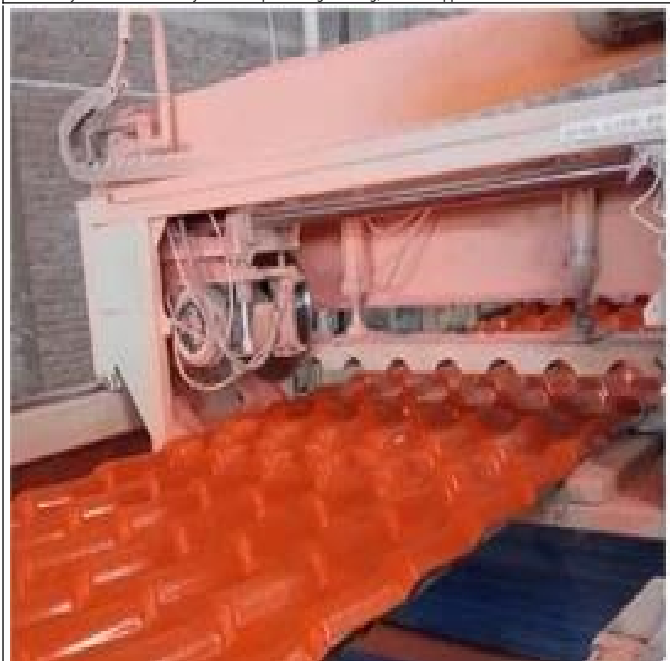
3. Then through the mold pressure, elastic molding, cooling, through the traction machine slowly introduced
