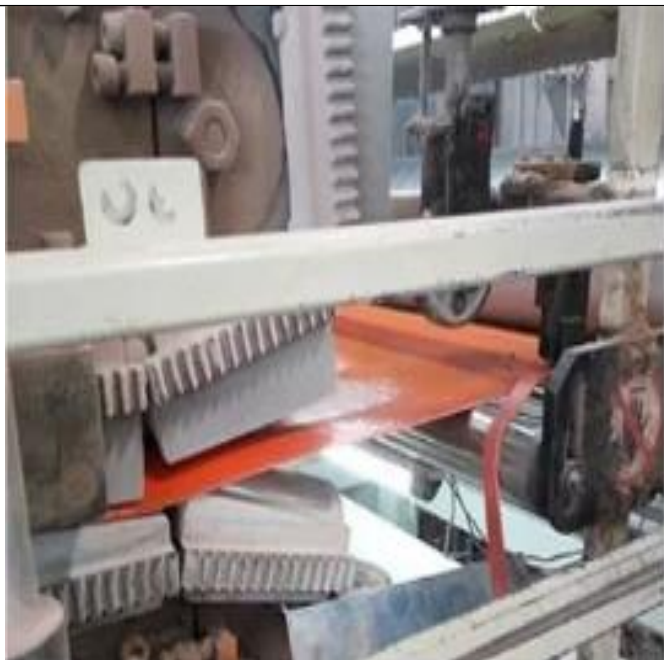
2. The mixed raw materials are pre-formed and heated to become flat tiles
