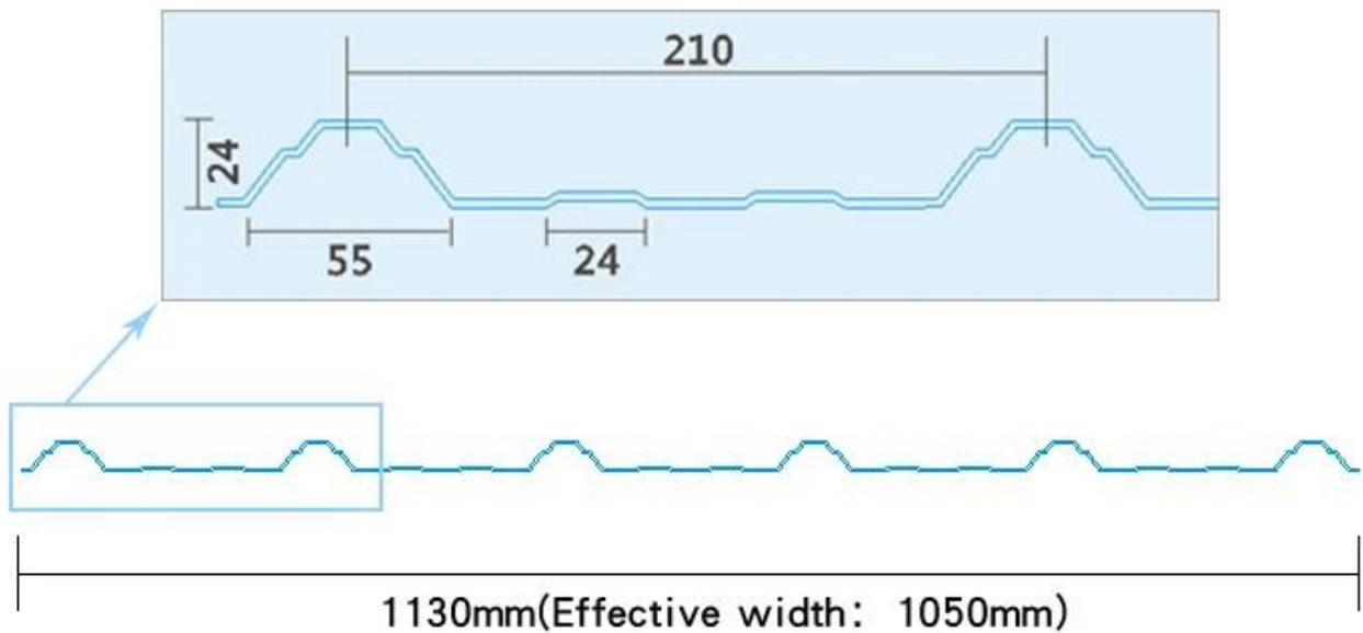
The product is a two-color three- or three-color three-layer super weather-resistant anti-corrosion composite tile, and the surface layer material is ASA super weather-resistant engineering resin. In the middle is a poly-recorded vinyl resin with excellent toughness. The bottom material is white tough wear-resistant material to increase the space sense and brightness and wear resistance of the plant.
