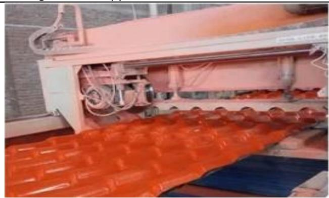
3. Then through the mold pressure, plastic the molding, cooling, through the traction machine slowly introduced
