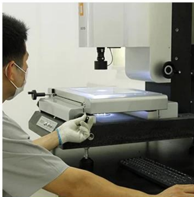
ASA SURFACE THICKNESS TEST
