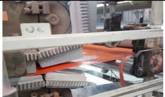
2. The mixed raw materials are pre-formed and heated to become flat tiles
