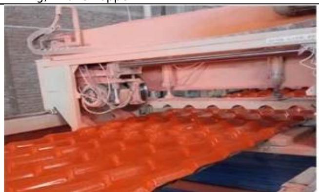
3. Then through the mold pressure, elastic the molding, cooling, through the traction machine slowly introduced
