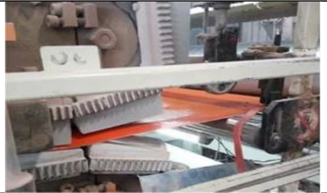
2. The mixed raw materials are pre-formed and heated to become flat tiles
